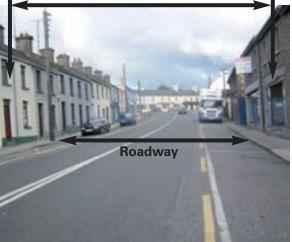
**Photograph 1** A street showing the extent of the roadway, including dedicated parking bays. The road is also shown and includes the roadway and the associated footways.
